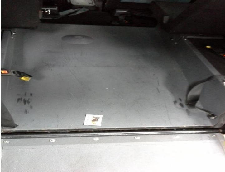
Acceptable, minor scuffs and scratches lowered floor
