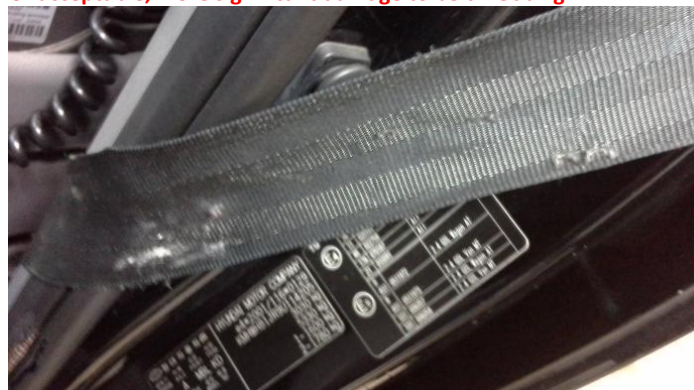
Unacceptable, more significant damage to belt webbing
