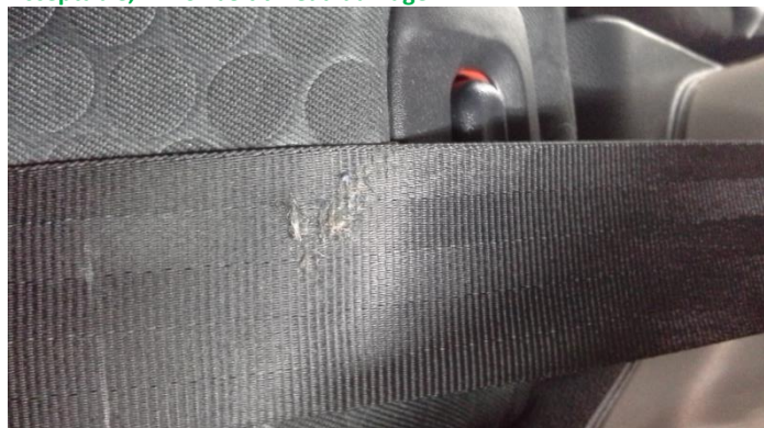
Acceptable, minor belt thread damage
